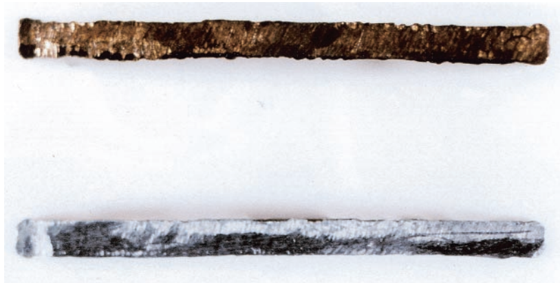
Fig 1. Cross-sectional view of pre-1982 (above) and post-1982 penny (below). The post-1982 penny demonstrates the thin copper coating overlying the zinc core.
