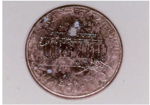
Fig 3. Penny obverse after endoscopic removal. Note corrosion of copper coating and exposure of gray zinc.
